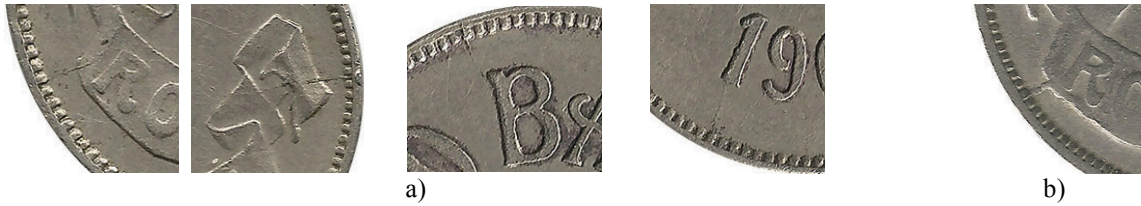
Figure 5. Various cracked dies error on 10 and 20 bani holed metal coin, issued in 1906
